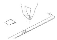
Press the RESET button with a small pin or clip.
